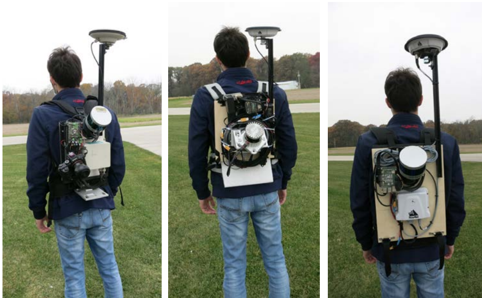
Figure 1. Prototypes for the three different backpack systems equipped with VLP 16 High-Res (left), Ouster (middle), and VLP 16 (right) LiDAR units.
