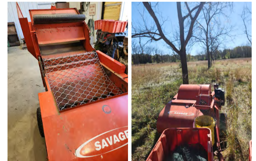
The acquisition of an oversized sizing chain (left) for the HTIRC's Savage pecan harvester considerably increased the speed of bulk harvests of black walnut, especially in seed orchards like the grafted select black walnut orchard at the Jasper-Pulaski state tree nursery (right).
