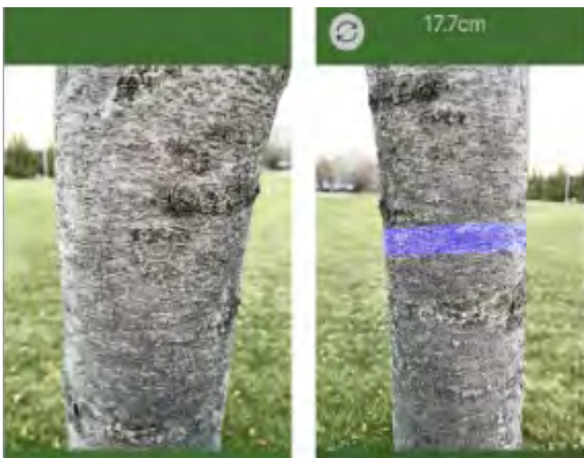
Figure 1. Measure tree diameter by tapping the tree image at an appropriate distance. To achieve accurate measurement, the tree bark occupies at least 70% of the screen width, as shown on the left image. Re-tap the image until the tree is clearly segmented. The ends of the red line should align with the boundary of the tree trunk, and the number (17.7 cm) on top of the right image shows the measured tree diameter.
