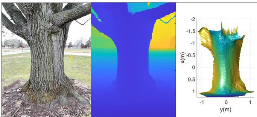
Figure 5. An example of tree reconstruction. Some vein information is missed in the 3D geometry. However, it makes the data smooth and is better for our diameter estimation.
