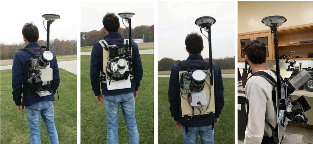
Figure 2. Prototypes for the four different backpack systems equipped with VLP 16 High-Res (left), Ouster (middle left), VLP 16 (middle right), and HDL 32E (right) LiDAR units.
