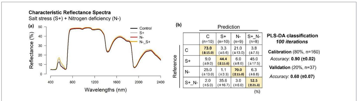
Figure 2. (a) Characteristic reflectance spectra of control, salt stressed (S+), nitrogen deficiency (N-), and combined salt and nitrogen stressed groups (S+\_N-). (b) A confusion matrix showing the results of the PLS-DA classification based on hyperspectral data to classify salt and nitrogen stressed groups. Yellow indicates correct classification.
