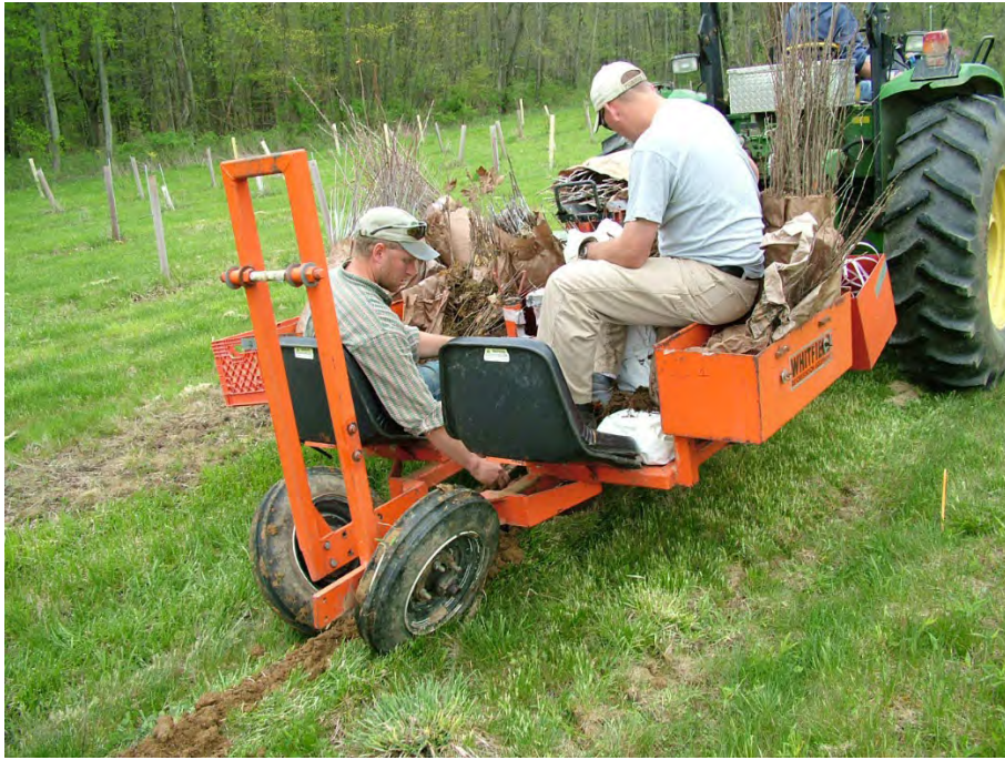
A tree planting machine and experience crew can plant thousands of trees per day.
