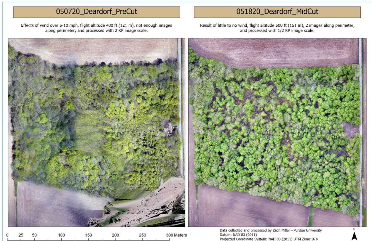
Figure 1: Difference between initial and revised flight planning on orthomosaic quality.
