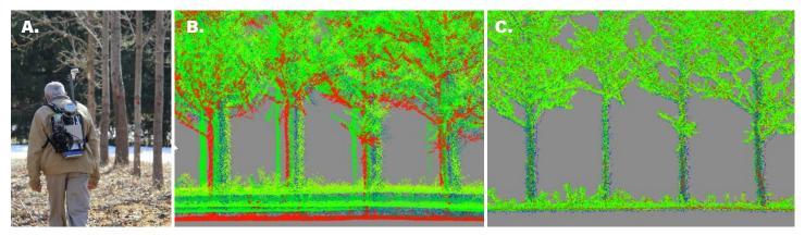
Figure 2. Backpack deployment in Martell Forest (a), and LiDAR point clouds before (b) and after (c) trajectory enhancement.
