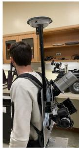
Figure 2. Prototypes for the four different backpack systems equipped with VLP 16 High-Res (left), Ouster (middle left), VLP 16 (middle right), and HDL 32E (right) LiDAR units.
