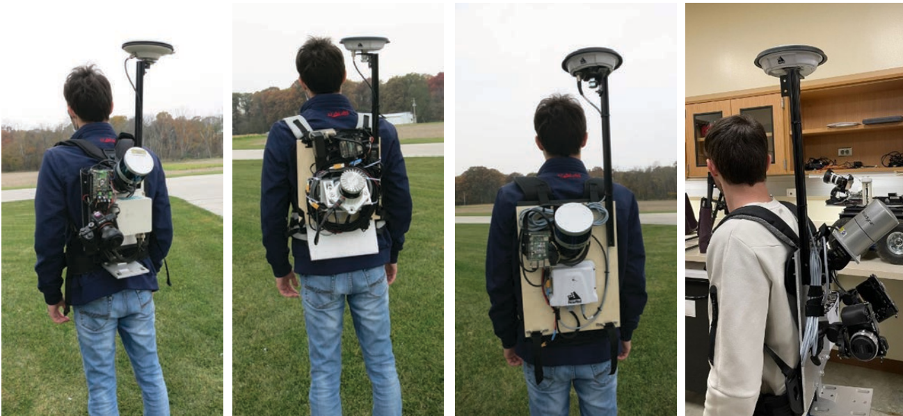
Figure 2. Prototypes for the four different backpack systems equipped with VLP 16 High-Res (left), Ouster (middle left), VLP 16 (middle right), and HDL 32E (right) LiDAR units.
