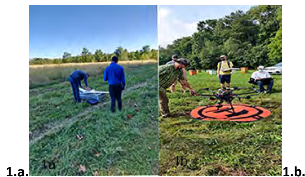
Figure 1.a. A fixed wing UAS platform, b. Multi-rotor platform experimented to derive 2D images of a red oak plantation in the northern part of Martell Forest, Indiana.
