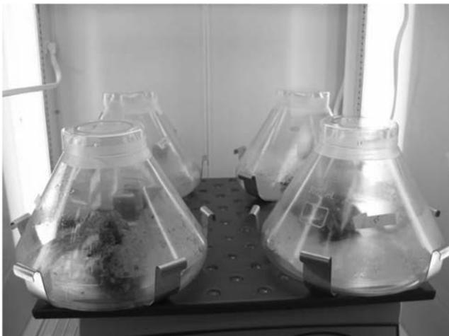
**Figure 1.** Three-liter polycarbonate Fernbach-style flasks on a rotary shaker that have been modified to create a larger opening to accommodate *Juglans nigra* L. shoot cultures.
