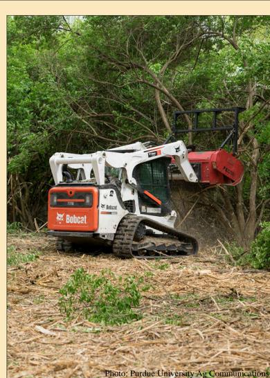
Mulching heads disturb soil and deposit a layer of woody mulch
