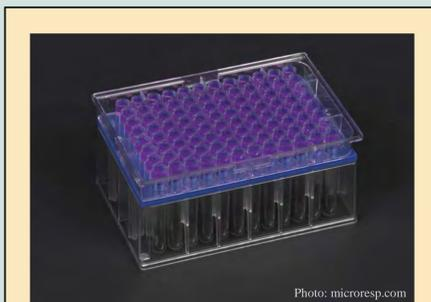
MicroResp system used to measure soil microbial catabolic activity
