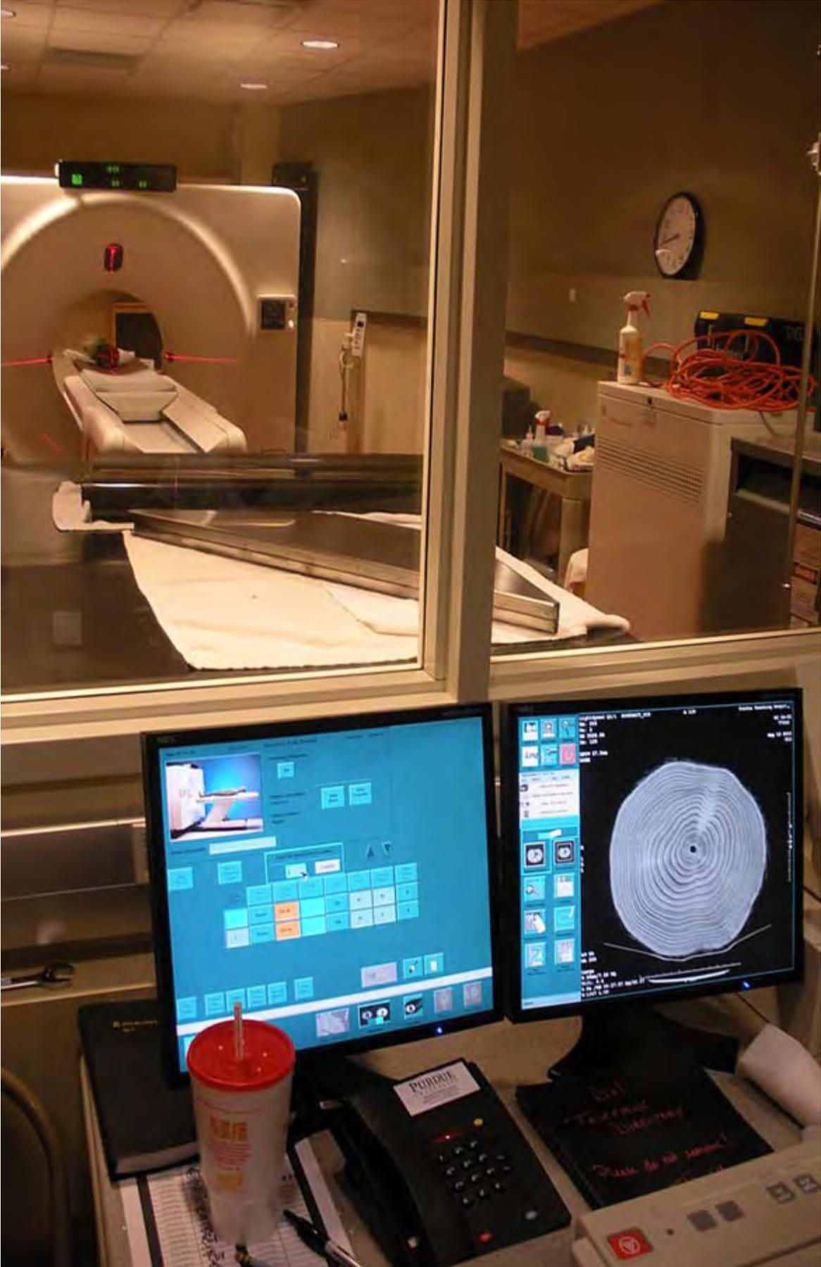
Figure 3. White oak log being scanned
