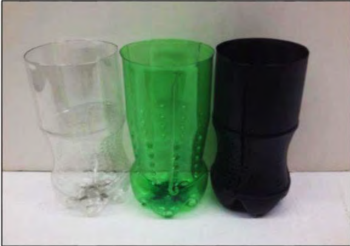
Figure 4. Comparison of three bottle opacities (clear, green, and black; left to right) and three spiral control techniques (control, interior-ridges, and side-slits; left to right).
