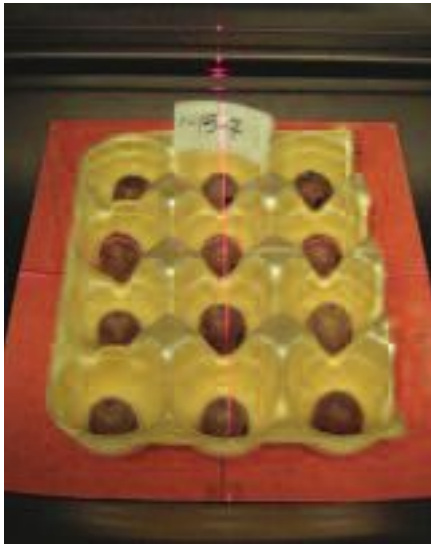
Figure 1. A sample of acorns, arranged vertically in indented carton, ready to be X-rayed. Photo by Rosa C Goodman
