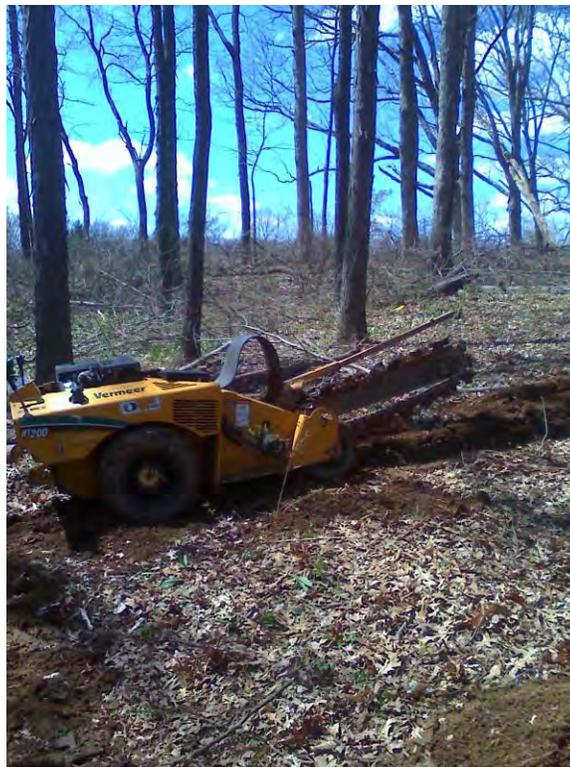
The trencher used to sever belowground roots sits within the midstory removal treatment at our drier site, prior to planting in the spring of 2009.
