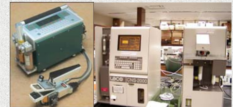
Figure 3. Equipment used in this study. On the left, a LI-6400 portable photosynthesis system. On the right, a LECO-2000 CNS analyzer.
