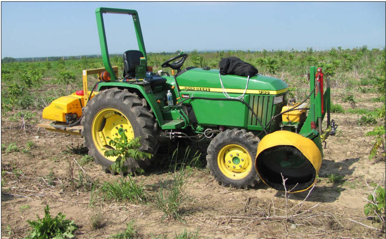
Figure 3.—Tractor-mounted control drop applicator with shield to control drift; this system is suitable for application of nonselective post-emergent herbicide. (Photo by J.W. Van Sambeek, U.S. Forest Service)
