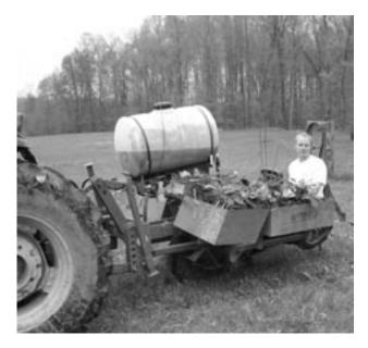
*Figure 1.* Tractor-hauled coulter with trencher and packing wheels, also equipped for herbicide application.
